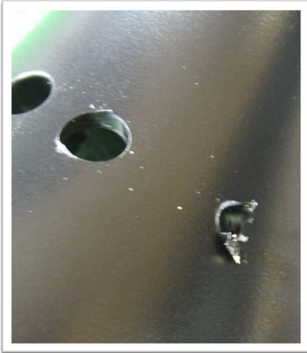
Holes with excess plastic
